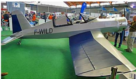
A light design permits Jörg's design objectives. "Due to the light weight of the structure we were able to include all the ingredients for a high performance aircraft: outstanding aerodynamics, a strong engine with a big, efficient propeller, a short and aerodynamic landing gear, as well as effective flaperons."
