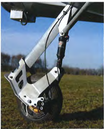
Below right Trailing arm main gear with oil-air damping units from a mountain bike
